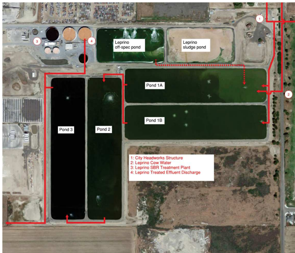
Figure 3.3 City Wastewater Treatment Facility Process Flow Diagram
